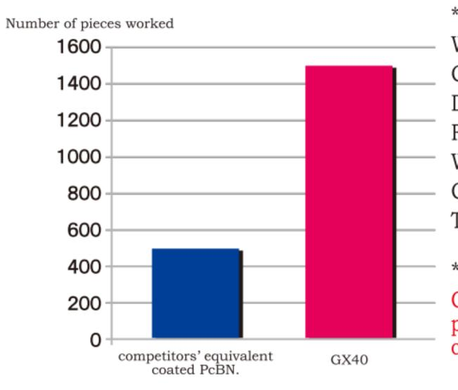
\*\* Test Parameters \*\* Work material: SCM415 (62HRc) Cutting speed vc: 130m/min. Depth of cut ap: 0.15mm.
