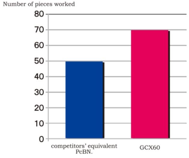
\*\* Test Parameters \*\* Work material: FCD450 Cutting speed vc: 200m/min. Depth of cut ap: 0.5mm. Feed f: 0.20 mm/rev. Wet mode
